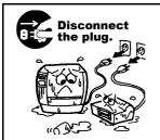
If foreign objects (metal fragments, water, liquids) enter the machines, first turn off the power switches and disconnect the power cord plugs from the outlet, and then contact your authorised TOSHIBA TEC representative for assistance. Continued use of the machine in that condition may cause **fire** or **electric shock**.
